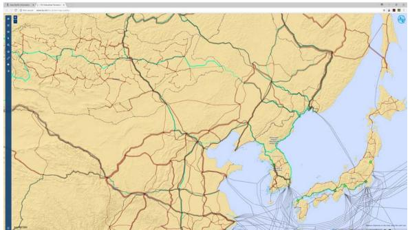
Source: AP-IS Transmission Map at <a href="www.itu.int/itu-d/tnd-map-public/">www.itu.int/itu-d/tnd-map-public/</a> (accessed on 21/08/2018). Blue line indicates Asian Highway routes; green dots are IXPs; barbed line indicates Trans-Asian railway routes; dark red is the transmission links.
