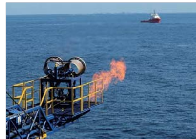
Flare from offshore production test
