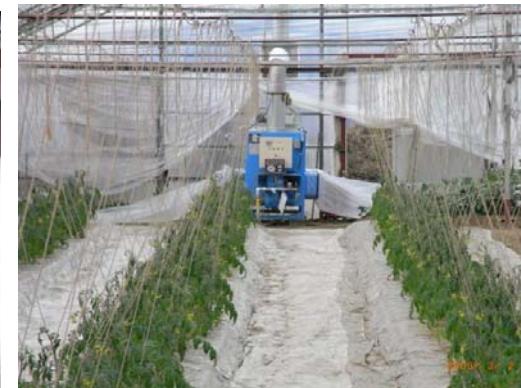
DME fuel used warming machine for the green house cultivation. Exhaust gas used to promote the plant.
