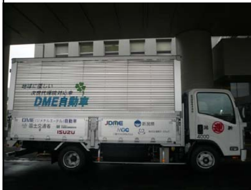
Development of DME Trucks for Public Road Test by Commercial Use in 17th, Nov. 2009
