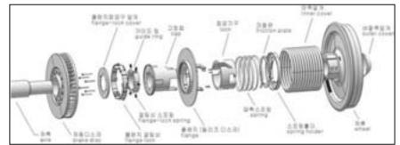
Figure 3.10 Automatic Variable Gauge Bogies
