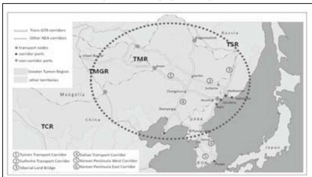
Figure 3.9 Break of gauge in GTI region
