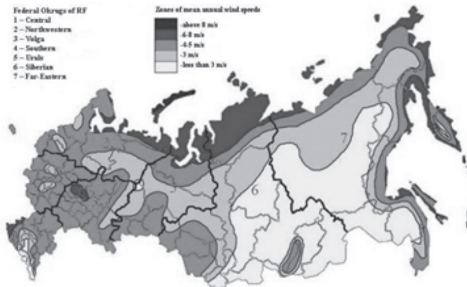
Fig. 5 - Zoning of Russia's territory in terms of the index of mean annual wind speeds
