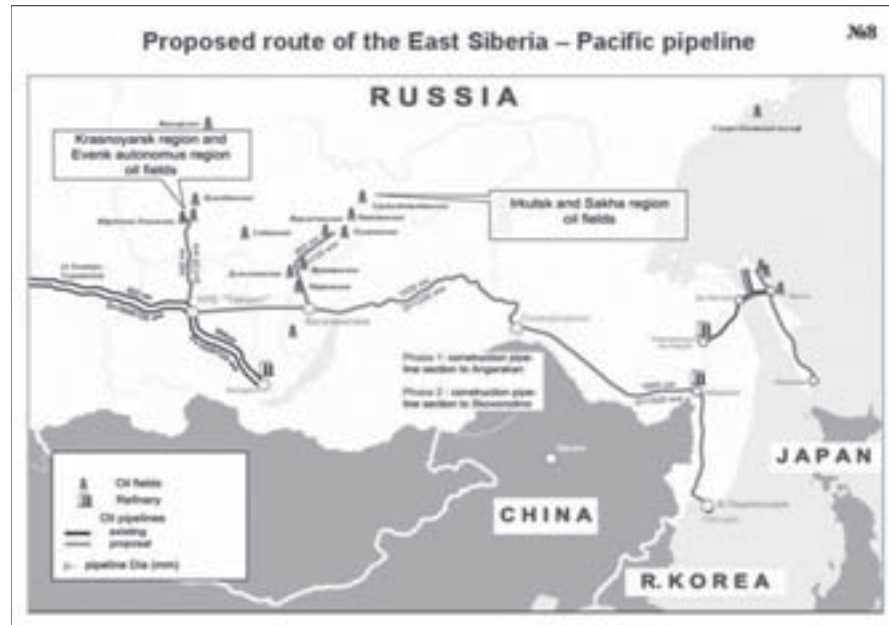
Figure 3 The Two-Phase Plan for the ESPO Pipeline
